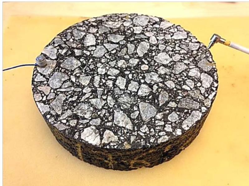
**Figure 3: The accelerometer attached to the specimen and the impact hammer**
