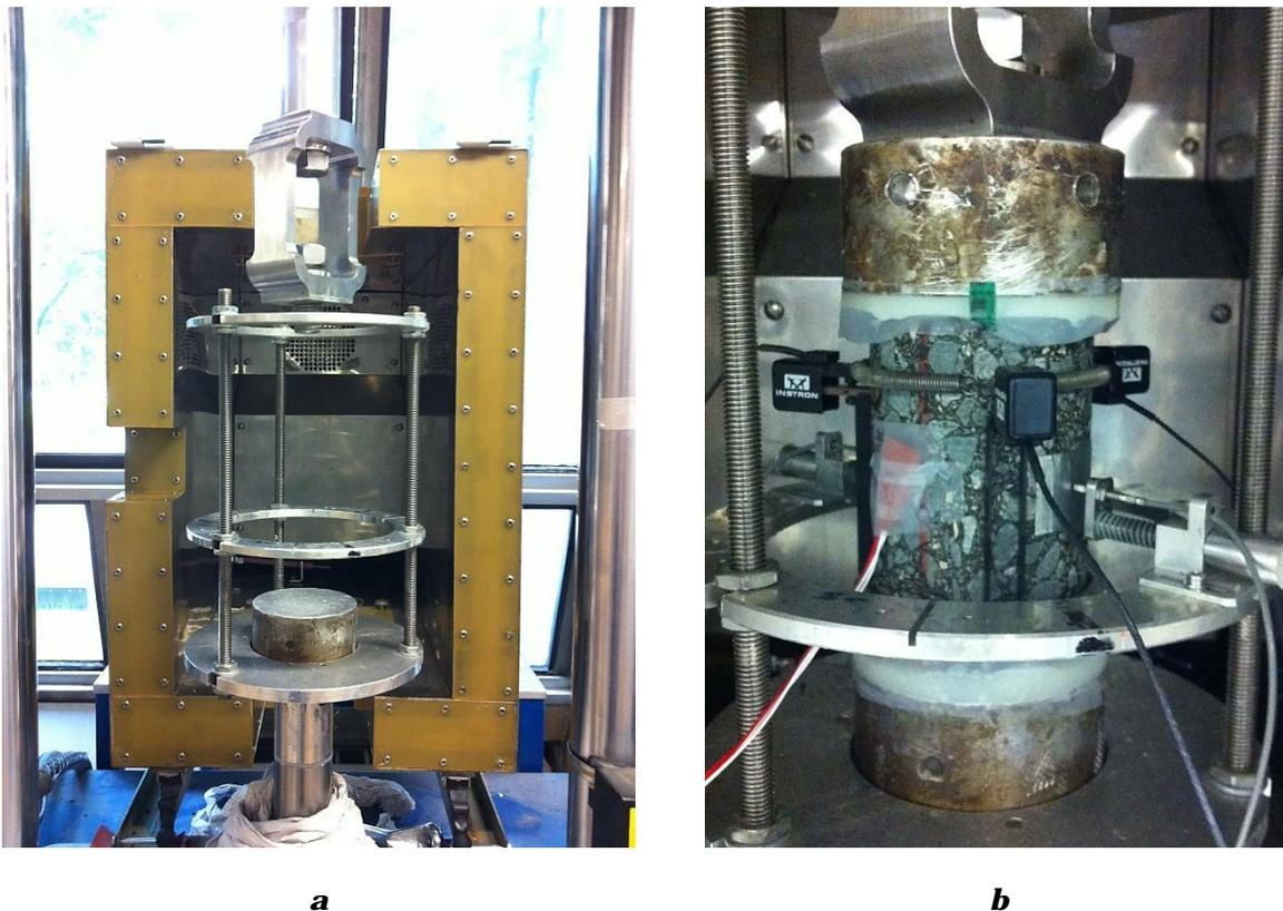
**Figure 2: Example of equipment and test set-up to perform conventional cyclic loading (a) and a detailed set-up of a specimen (b). The photos are taken at ENTPE, University of Lyon**
