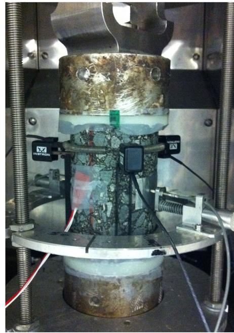
Fig. 3 Test set-up of the tension–compression complex modulus and complex Poisson’s ratio measurements
